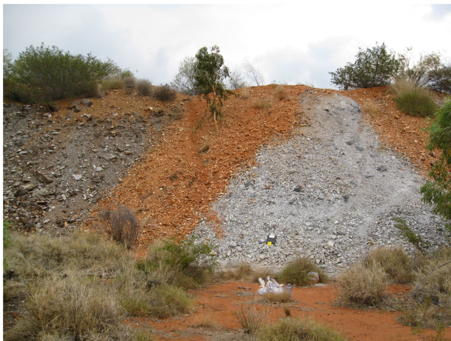
Fig. 2. Fine grained and rapidly weathering material (dark grey on left and light grey on right). Both materials are hostile to plant growth due to high salt content. The red-brown material is soil and saprolite and supports vegetation. (For interpretation of the references to colour in this figure legend, the reader is referred to the web version of this article.)
