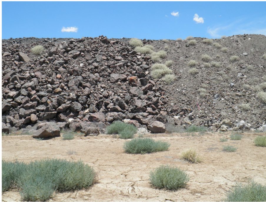
Fig. 1. Waste rock with very large particle size (left hand side) and less large on right hand side. Monitoring has found the materials to be erosionally stable but with little capacity to support plant growth due to the lack of fine material – the limitation being water holding capacity of the material.
