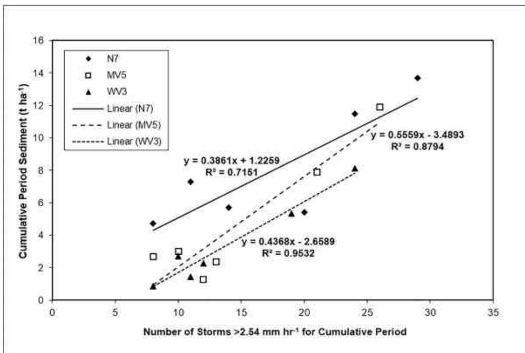
Fig. 15. Cumulative period sediment versus cumulative period number of storms greater than 2.54 mm h<sup>-1</sup> produced the strongest linear relationships of sediment to rain event.
