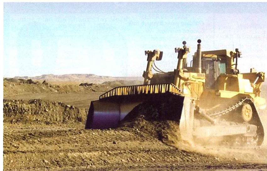
Using specially developed software and GPS guidance systems on dozers, BHP Billiton's La Plata mine restored mined desert lands efficiently and cost-effectively.
