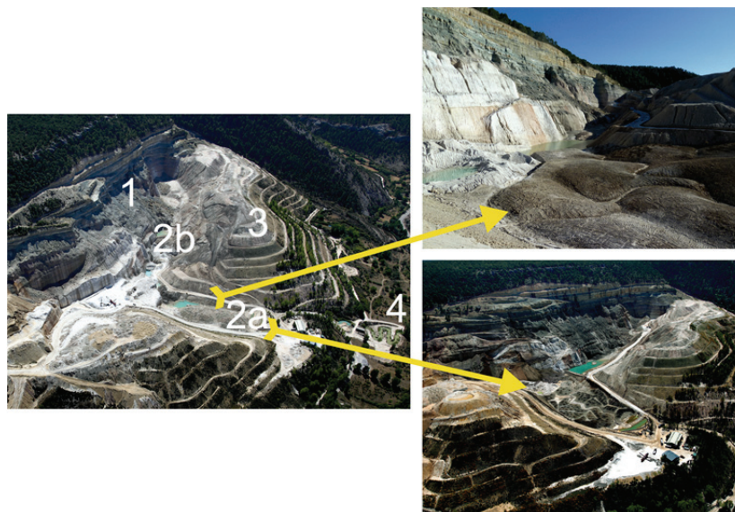
Figure 9. The María José mine created a man-made valley (2 at the left image) between the highwall (1 at the left image) and the outslope-terraced waste dump (3 at the left image). This landform has no local physiographic analogy. We proposed reshaping that valley to one more compatible with the nearby natural ones by using the GeoFluv method. The right images show details of the first phase of construction (zone 2a at the left image), with a main meandering channel (B type of the Rosgen classification). The 2b zone will be reclaimed following the same pattern.
