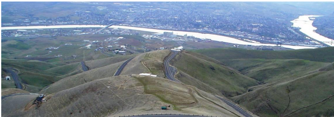
Figure 3. High gradient channels have formed on either side of the ridgeline in the center of the image (Idaho). Note the characteristic zigzag channel pattern and the absence of rills and gullies in the subwatersheds draining to these ephemeral channels.
